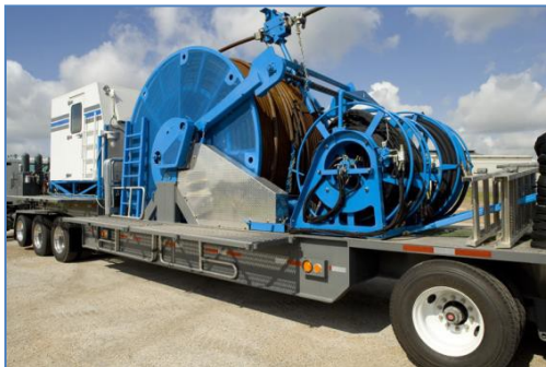
Figure 1 Coil tubing truck carrying a large spool of 2" tubing with the injector head (right side). Courtesy Stewart and Stevenson Inc. 2013
